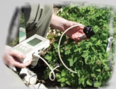
LED's have the advantage of being rugged, emitting low levels of heat, and of rising to full intensity very rapidly (typically microseconds) after being switched on. This feature eliminates the inaccuracies of  $F_o$  measurement and the constraints on speed and
