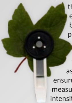
The leaf or needle rests on a foam pad whilst in the clip in order to minimise damage to the structure of the leaf. The shutter plate should be closed to exclude light from the sample during dark adaptation.
