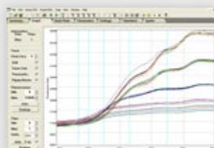
PEA Plus provides a comprehensive tool for in-depth analysis of data recorded by the Pocket PEA chlorophyll fluorimeter. Several different data presentation techniques have been combined in order to effectively demonstrate subtle differences in the fluorescence signature of samples which could be indicative of stress factors affecting the photosynthetic efficiency of the plant.
